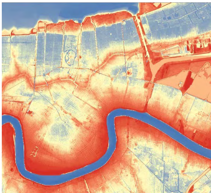
A LIDAR elevation model of New Orleans shows areas above sea level in red tones (up to 10 or 15 feet, except for the artificial levees) and areas below sea level in yellow to blueish tones (mostly ranging from -1 down to -10 feet). (Richard Campanella / FEMA)
